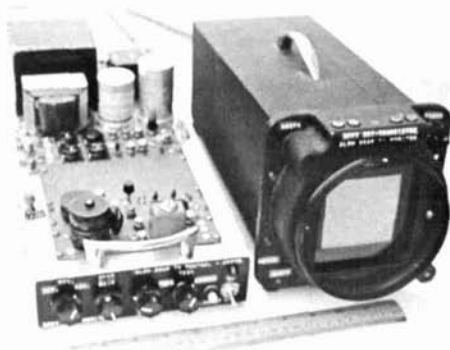
Solid-state sstv monitor using a 5FP7 tube. The photos of the ID chart and the authors were made from W3EFG's camera and this unit.
